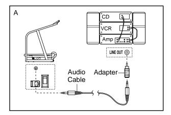
B. Plug one end of the audio cable into the jack on the side of the trainer near the power cord. Plug the other end of the cable into the included adapter. Plug the adapter into an RCA Y-adapter (available at electronics stores). Next, remove the wire that is currently plugged into the LINE OUT jack on your stereo and plug the wire into the unused side of the RCA Y-adapter. Plug the RCA Y-adapter into the LINE OUT jack on your stereo.
